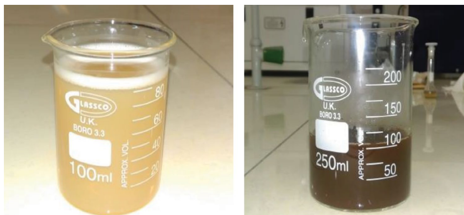
Fig.1. Color change of solution due to the synthesis of silver nanoparticles.
